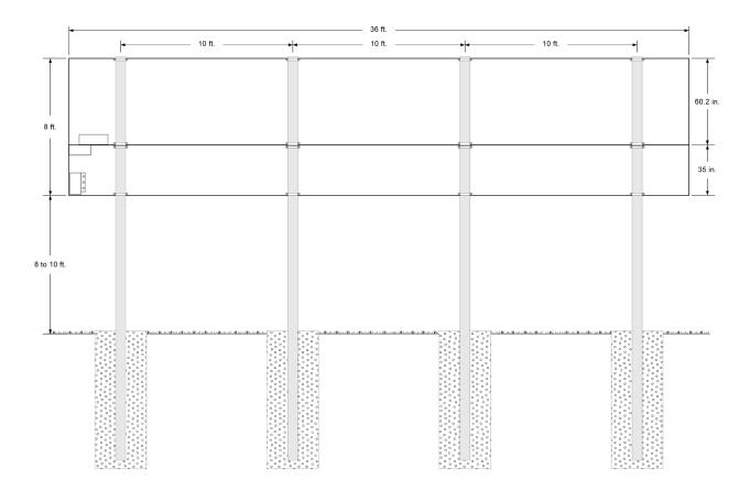
Once you have verified the positions of the posts and the size of the footings, you are ready to dig your holes, pour your concrete, and set your posts. There are several techniques for ensuring proper alignment of the posts. Typically installers will construct a temporary wooden support frame to hold each post in place while the concrete sets. Having plumb posts in the proper position is the key to a smooth mechanical installation.
